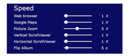
These settings can define the speed in scrolling with the eyes in the various types of grids. The speed is defined in multiplying factor compared to default: for example, 5X means 5 times quicker than default.
