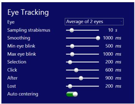
This section is only necessary if you have selected input mode = eye tracker. It will enable you to fine tune the eye tracking mode in Gazespeaker.
